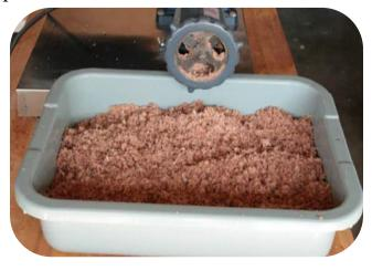
The grinder is a large #32 manual ChopRite with a 1 ½ horsepower motor in place of the handle and fitted with a "bean" plate that has 3 very large oval holes.
