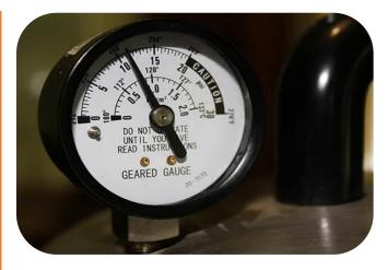
When the processing time is over, turn off the heat and leave the canner in place until it is back down to o pounds of pressure. Once it's at o pounds, remove the weighted gauge to allow the last little bit of steam to escape before unscrewing the lid.
